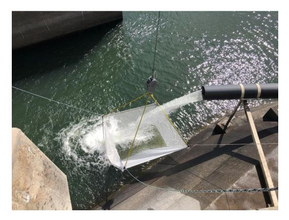
Net pen improperly positioned under bypass discharge, too far out of the water. This problem increased as testing progressed, lowering the net resulted in it being pushed around out of position. Slings that were too short also made it difficult to position it as far into the water as desired.
